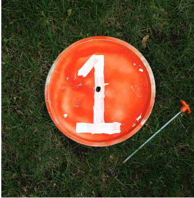
Figure 2-6: GCP Marker Used for This Study
